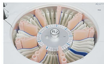
Reagent Tray 2~8°C cooling for 24 hours.
