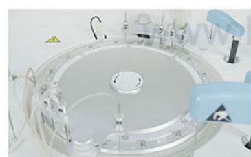
Reaction Tray 37±0.1°C, water bath.
